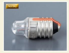
**HL-D3** can accurately sense the shapes of the thread and black insulation of a miniature bulb.
